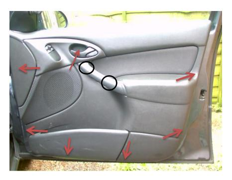
Remove 7xscrews from door card, take out 2x 7mm bolts inside the door handle circled, (you have to prize the cover off)
