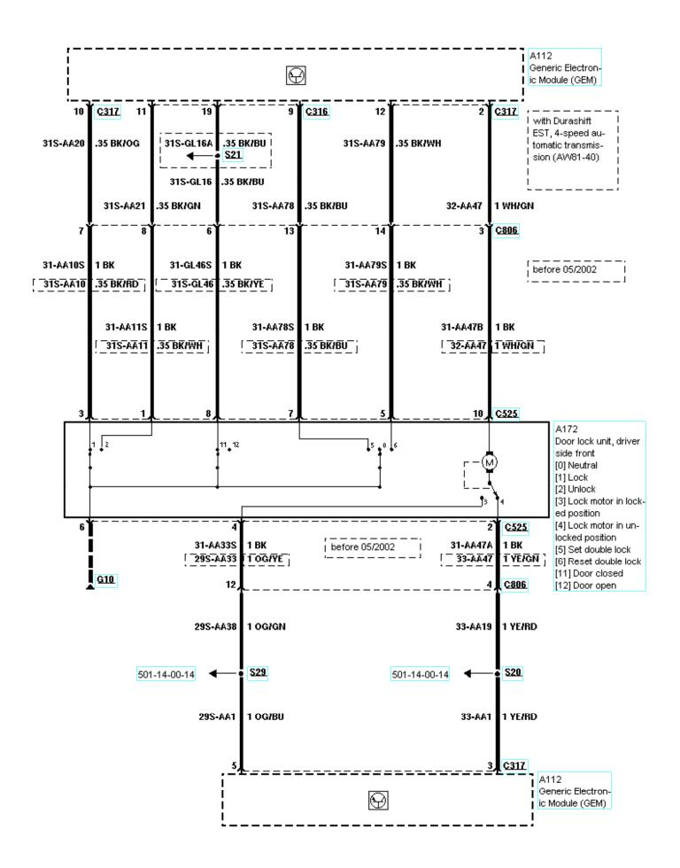
501-14-00-013, Handles, Locks, Latches and Entry Systems, With double locking, 5-door model
