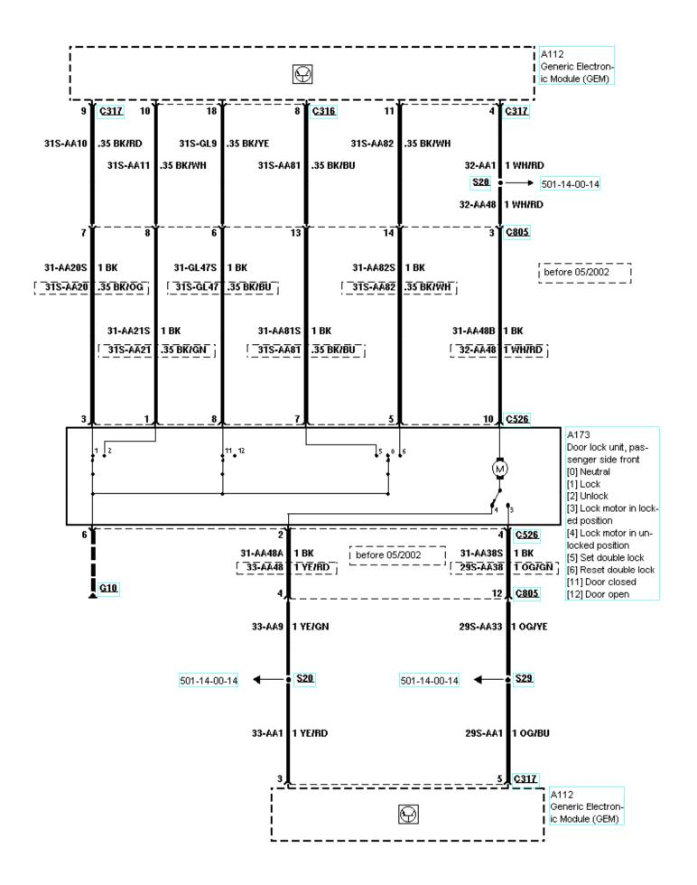
501-14-00-014, Handles, Locks, Latches and Entry Systems, With double locking, 5-door model
