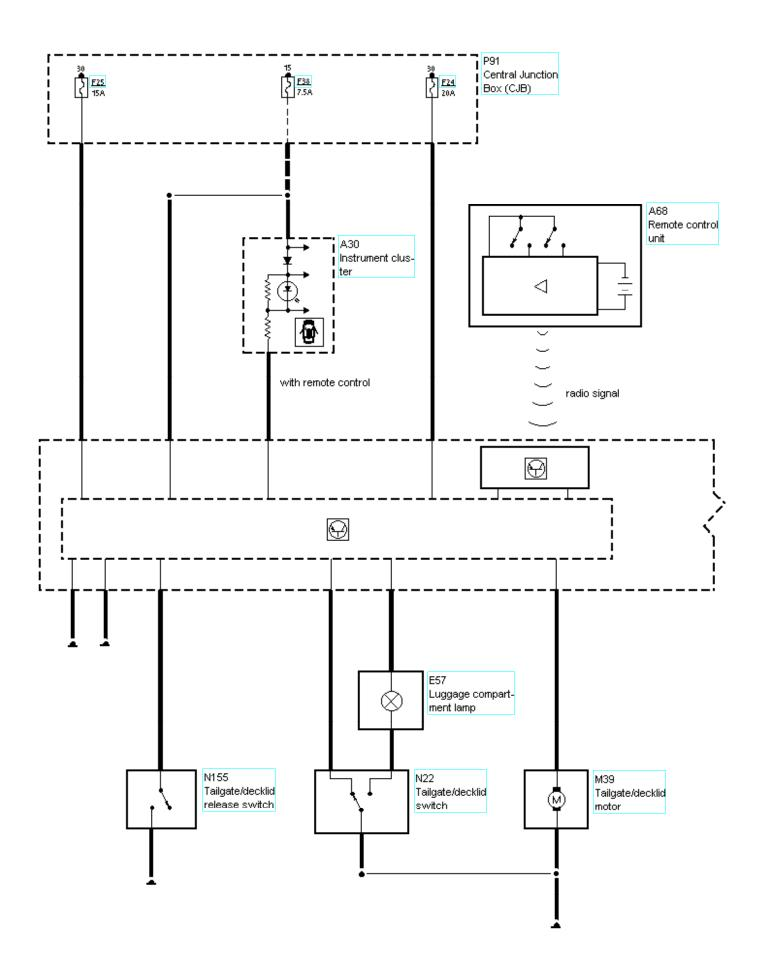
501-14-00-501, Handles, Locks, Latches and Entry Systems, Block diagram
