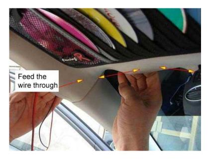
10. Feed the wire through the light opening and ensure you have spare so as to be able to remove the light at any later time.
