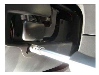
4. Remove the radio control stalk by inserting a small screwdriver into the slot on the rear of the unit and pressing gently on the clip, slide the stalk out of position and unplug the wire connector.
