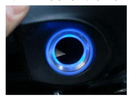
15. Push the circular LED PCB onto the illuminating ring ensuring the cable will not get snagged or twisted on any component under the steering wheel.
