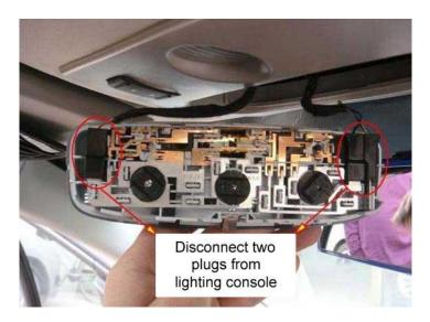
12. Reconnect the plugs to the corresponding connectors – connect to the plugs which are *not* at the end of the loom.
