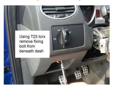
2. Remove retaining screw from beneath steering wheel using T25 screw driver.
