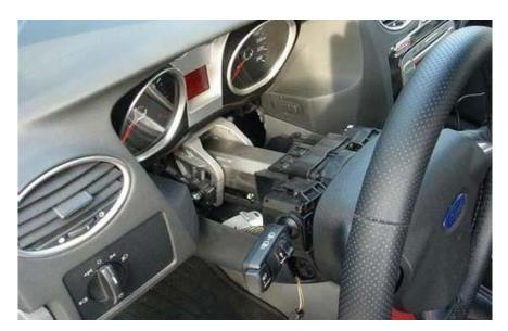
6. Remove steering column bottom facade, flexing out at the sides if necessary to clear obstructions.
