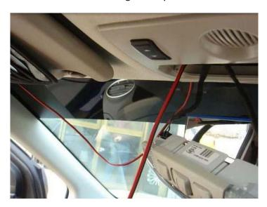
11. Disconnect the cable plugs from the light.
