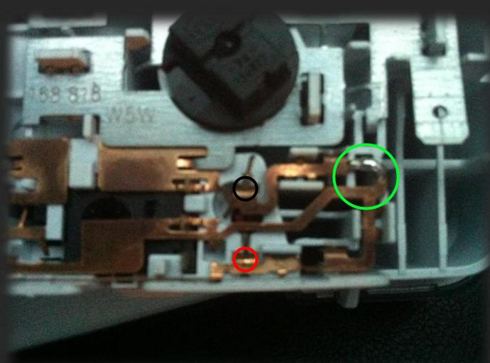
6. Now to complete the circuit you need to solder the section shown above circled in Green to attach the Negative feed.
