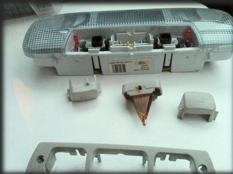
The two connectors on the LED's must have some protection to stop the two touching when passing through the holes circled Yellow above
