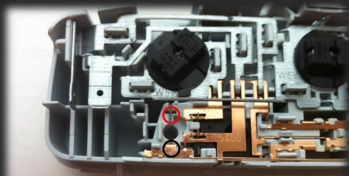
To attach the copper sections to the LED, apply pressure to the copper after lining up the V shaped section over the LED.
