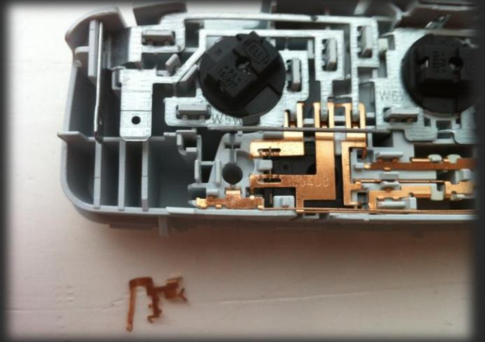
4. The LED's must be placed one in each hole, from the side shown
