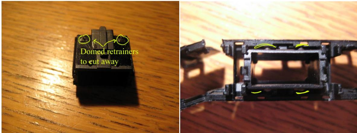
Once you have removed the blanking unit you simply push the ESP slider into place from the back, again a little flexing is needed.
