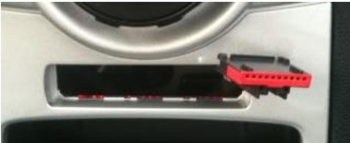
If you already have the ESP disable switch try fitting it and pressing it for 2 seconds to check your car can disable it's ESP.
