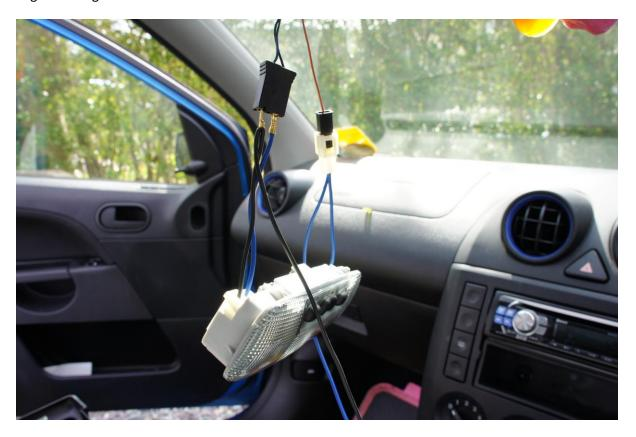
Now the wiring is in place you can choose to take this time to ensure that the light is working correctly.
