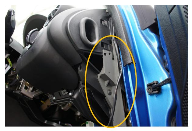
The plastic part circled in yellow can be removed by removing the screw this will allow for the loom to exit the dash neatly.
