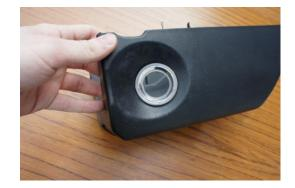
The next step is to install the lower cowel and ignition ring into the car, ensure that the led ring is located over the ignition barrel then offer up the steering cowel and then secure by pushing the other part of the ignition ring over the barrel. Ensure that the wiring doesn't get trapped behind the cowel when running the loom down the steering column and into the dash.
