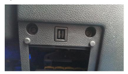
With these screws removed the panel can now be pulled away, the panel has 3 fixings points at the very bottom edge of and then on the right hand side next to the door rubber
