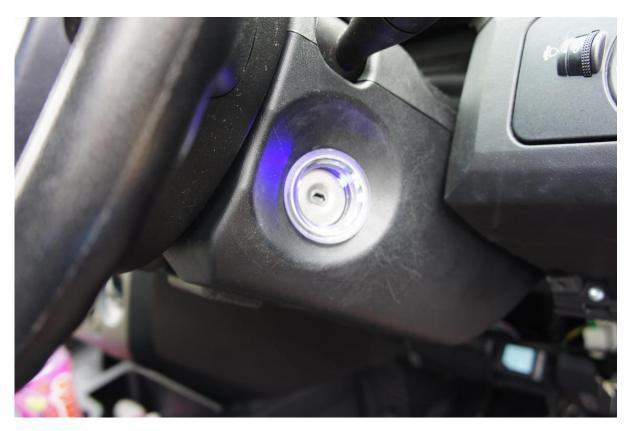
Now that the ring is secured into the steering wheel, the loom needs to be run through and up to the interior light.
