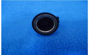
(False bulb holder removed to allow extraction if the 12 volt socket)
