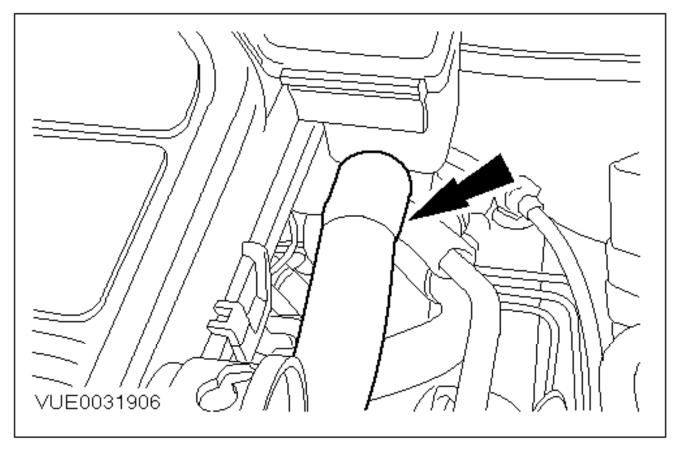
**c** 2. Disconnect the positive crankcase ventilation (PCV) hose from the air cleaner.
