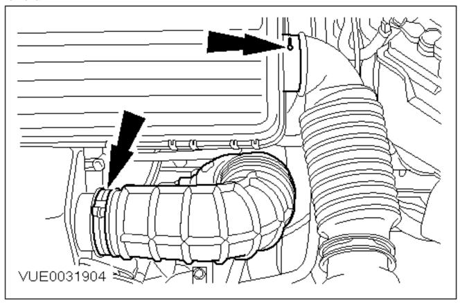
• 1. Disconnect the air cleaner intake and air outlet pipes from the air cleaner.
