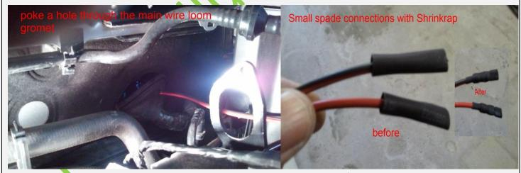
Connect Wires and clip diagnostics plug back in, clip cover back in place and re fit T20 hex screw .Replace glove box, Aircon pipe i needed to use long nose pliers to grip the side pipe and pull the clips back in place as there is no way of getting your hand behind and pushing it back on to the glove box.
