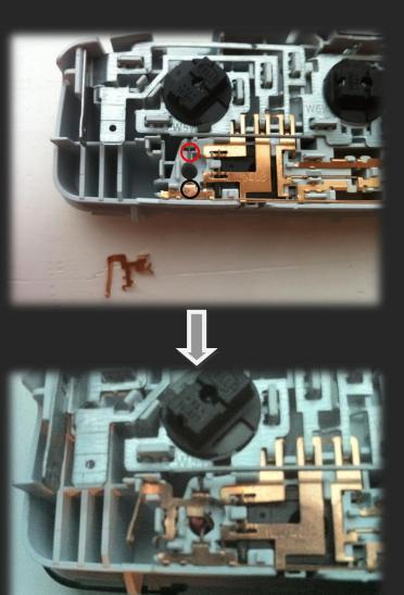
To attach the copper sections to the LED, apply pressure to the copper after lining up the V shaped section over the LED.
