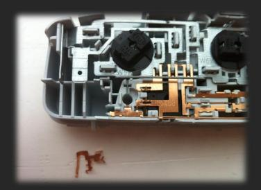
4. The LED's must be placed one in each hole, from the side shown
