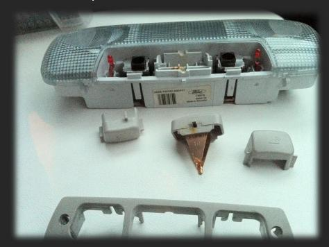
The two connectors on the LED's must have some protection to stop the two touching when passing through the holes circled Yellow above 5. To connect the LED's into the circuit, you must remove the sections of copper around each hole as shown below. The longer end to the LED (positive) must be connected to the side marked RED and the shorter (negative) to the side marked BLACK.
