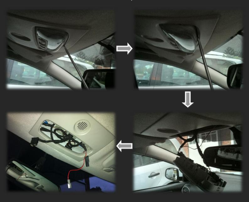
3. Disassemble the unit into pieces, then drill two  $3.5-4~\mathrm{mm}$  holes in the part circled red to line up with the holes circled yellow
