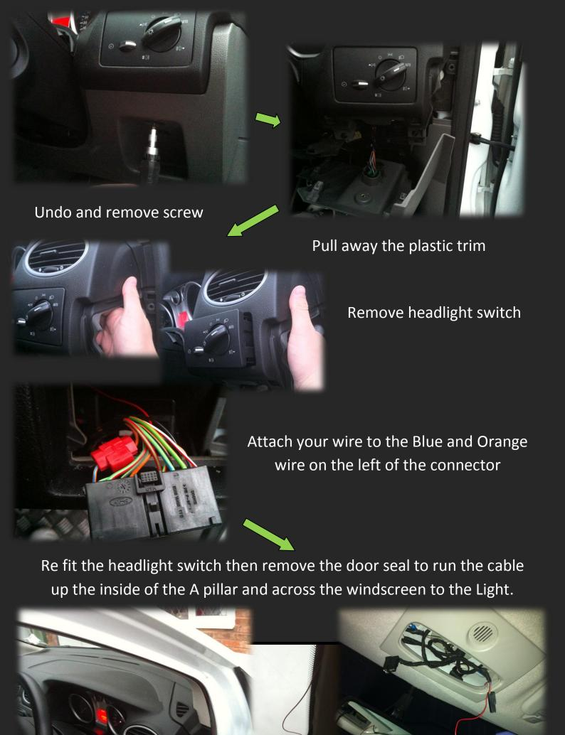
You should now connect the spade connector end of the wire to the pin on the light unit as shown, then now the LED's should come on with the Sidelights and Headlights, also works with Auto lights.
