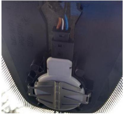
Now that you have wires all fitted and sensor fitted. You need to connect your new lights switch, if you squeeze the coin tray on drivers side it pops down revealing the cars pc connector for later on but above you can push the clips and pry the switch out, just swap out the switch and push back in. you can leave coin box down as you now need to connect up your pc with forscan to activate
