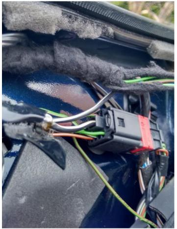
As you can see here you need to tap into the black/white wire and solder your new one into it, I have only spliced mine and wrapped wire around the other wire and with duct tape. As you can see lantt has soldered his, much better for a good connection I just doubted it working so wrapped it.
