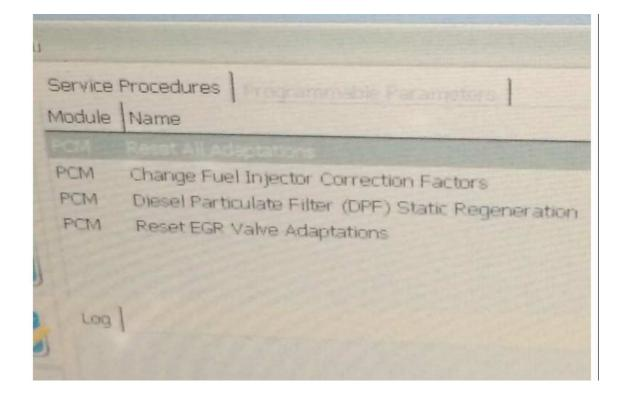
This will start a static regeneration and requires the engine to be running. You will need to follow the instructions on screen in order to complete this service process. This service process allows you also to complete calibration of injectors, EGR parameter resets and others depending on the car.
