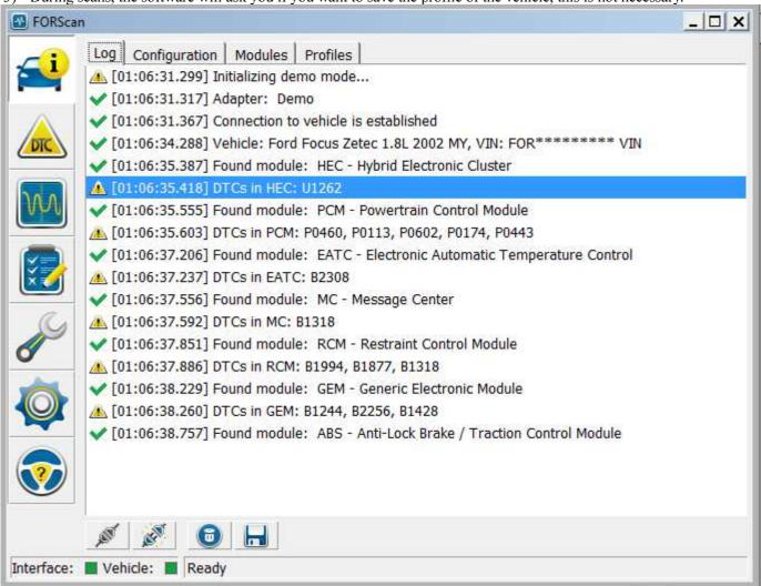
4) The software now shows you which modules it has communicated successfully with (a green tick), any error codes stored under that module are shown below it.
