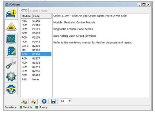
5) As you can see here, there is an error under all modules but the ABS. If you want to access the error codes, you can click the yellow DTC (in a triangle icon) to review further. Clicking on any error code will then extend the information, it will show you the error code, the module affected and the definition of it.
