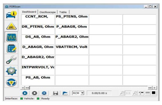
You can see the values on there which will populate when the car is running. For example, you may see the PS\_AB (Passenger Side Airbag) shows 2.8 OHMS. Then DS\_AB (Driver Side Airbag) may report 6 ohms. This shows that the value is too high, and is probably shorting out or has high resistance from a bad connector. You can see on the Table screen, the PID, the value and its plain english name (easier to navigate).
