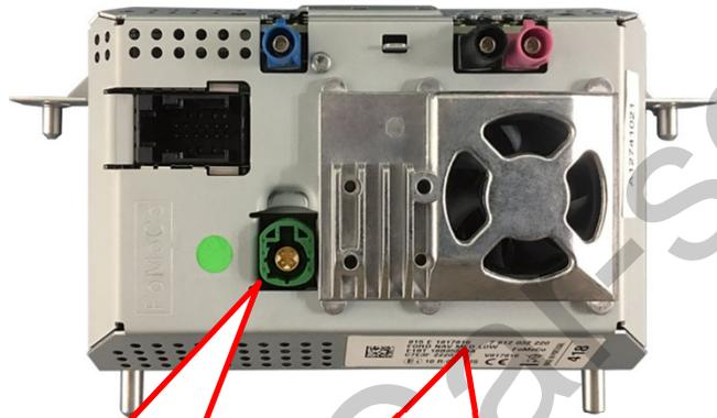
**SOCKET FOR REAR VIEW CAMERA CONNECTION**
