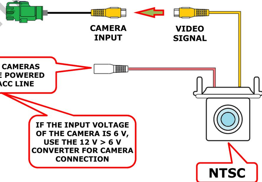
**12 VOLT CAMERAS SHOULD BE POWERED FROM ACC LINE**
