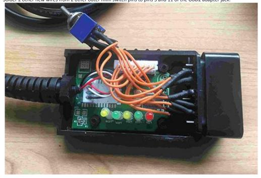
Check the work (it is very important to do not mix CAN-L and CAN-H wires up!) and assembly the ELM327 OBD2 adapter, mark the MSCAN bus and HSCAN bus position on the device box to avoid confusion.
